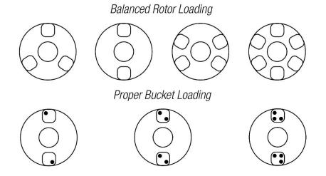
15 mL / 125 mm tubes may be spun in the standard HORIZON 24 Flex buckets, but must be loaded as follows:
