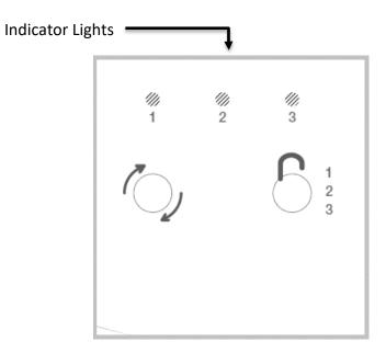
Each number represents a preset cycle. Above each cycle number is an LED indicator light. The LED indicator light changes to indicate the cycle currently selected:
