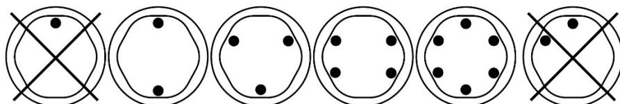
*Buckets can be placed around the rotor in any of the rotor loading configurations shown.
