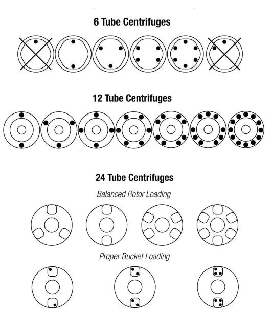
Buckets can be placed around the rotor in any of the rotor loading configurations shown. Each bucket must be loaded symmetrically with tubes as above.
