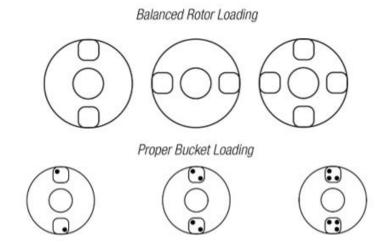
Buckets can be placed around the rotor in any of the rotor loading configurations shown. Each bucket must be loaded symmetrically with tubes as above.
