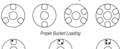
Buckets can be placed around the rotor in any of the rotor loading configurations shown.
