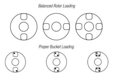
Buckets can be placed around the rotor in any of the rotor loading configurations shown.
