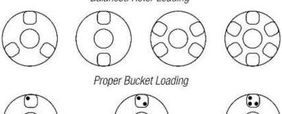
Buckets can be placed around the rotor in any of the rotor loading configurations shown. Each bucket must be loaded symmetrically with tubes as above.
