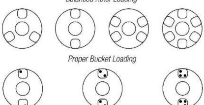
Buckets can be placed around the rotor in any of the rotor loading configurations shown.
