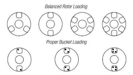
Buckets can be placed around the rotor in any of the rotor loading configurations shown.
