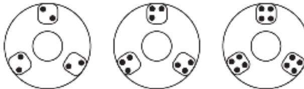
**When all six buckets are being used**, the rotor must be loaded in the following configuration **only**. Opposing buckets do not need to be filled but must be loaded in exactly the same way.
