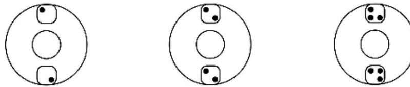
**15 mL / 125 mm tubes** may be spun in the standard HORIZON 24 Flex buckets, but must be loaded as follows:
