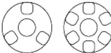
**When three buckets are being used**, each bucket must be loaded symmetrically in any configuration below:
