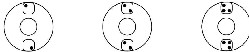
*Buckets can be placed around the rotor in any of the rotor loading configurations shown.
