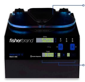
View RPM and remaining spin time on the digital display
