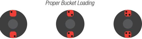
Buckets can be placed around the rotor in any of the rotor loading configurations shown. Each bucket must be loaded symmetrically with tubes as above.
