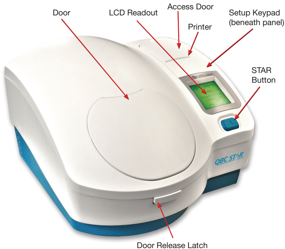
Figure 8 – QBC STAR Controls and Indicators
