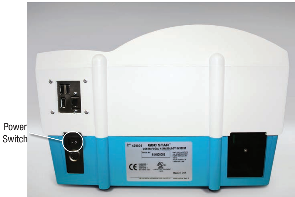
Figure 7 – Power Switch (toward left)
