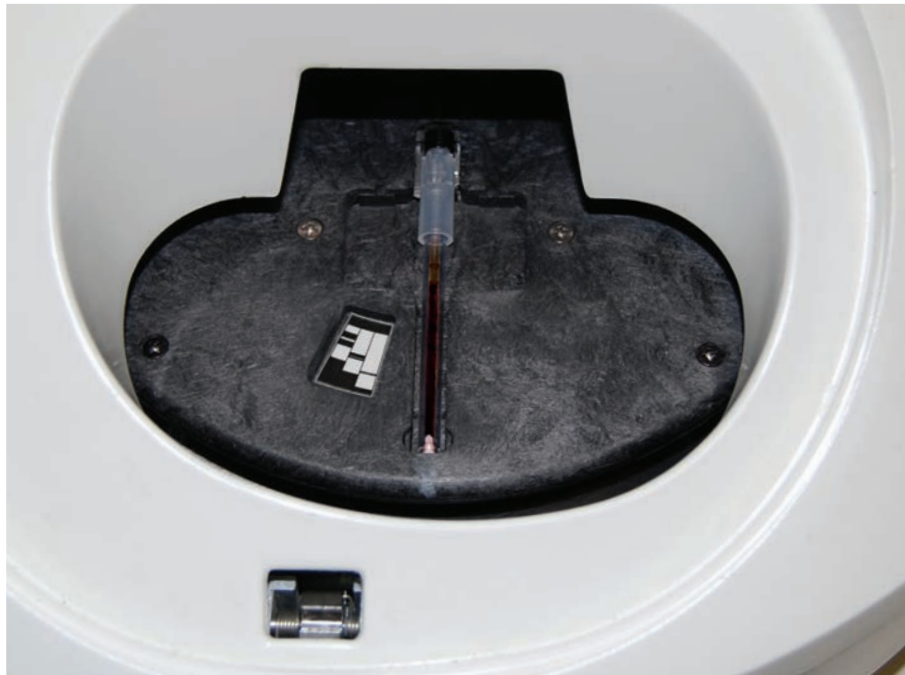
Figure 19 – Inserting the Tube into the Instrument
