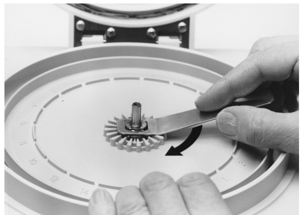
Figure 3-5. Tightening Rotor with Head Nut Wrench
