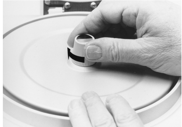
Figure 4-4. Tightening Knob of Rotor Cover.
