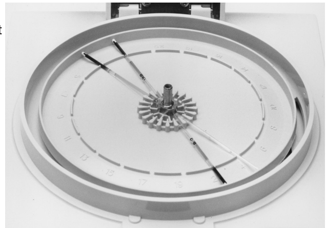
Figure 4-3. Typical Placement of Blood and Balance Tubes.
