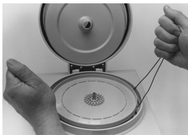
Figure 9-1. Prying Rotor From Motor Shaft with Removal Wire.
