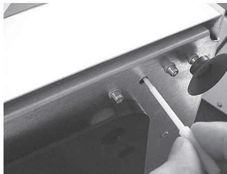
Calibration access hole
