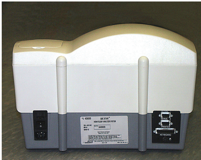
Figure 5 – Power Switch (toward left)
