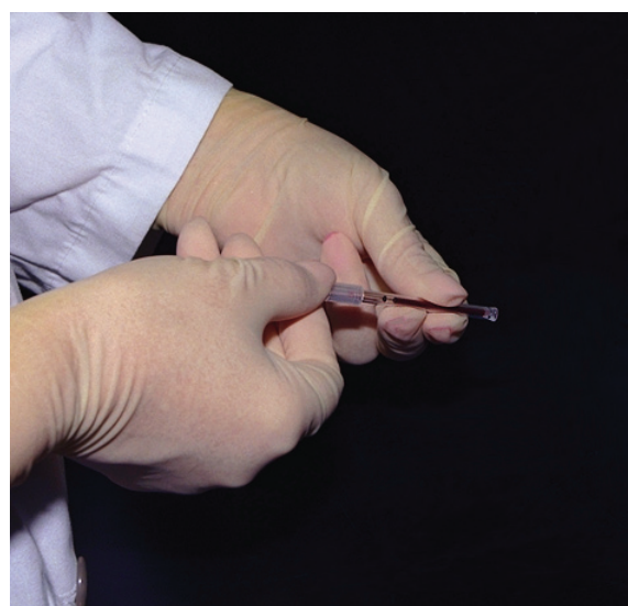
Figure 17 – Seating the Cap and Float
