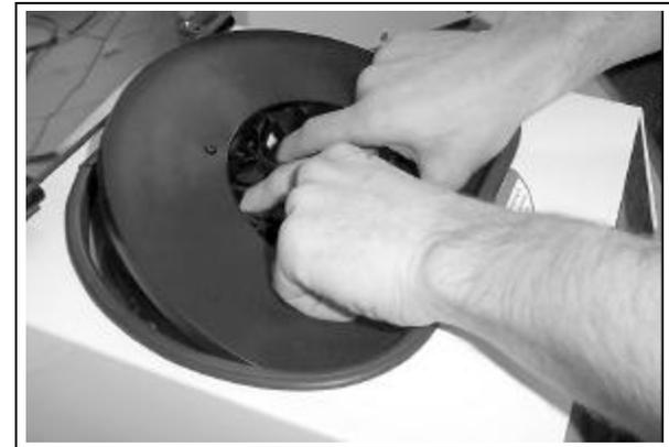
**Proper Rotor Position for Installation and Removal**
