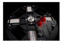
The TrueBond TriFLEX is a drop-in replacement for the discontinued BD Triac. Its unique rotor design spins flat microhematocrit and fixed-angle fecal, urine and blood tubes.
