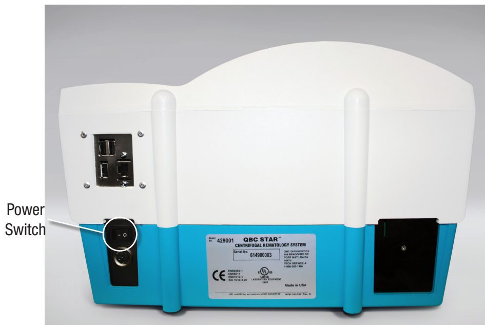
Figure 7 – Power Switch (toward left)
