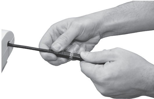
Figure 3-2. Connecting Power Pack Output Cable to Centrifuge Power Input Cable
