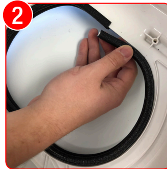
2 Starting at 12 o'clock position, apply the new gasket around the lid well; clip off any excess
