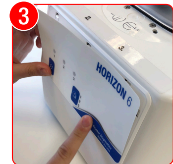
3 Replace the new front panel label, making sure that it is properly aligned in the channel on the molded panel
