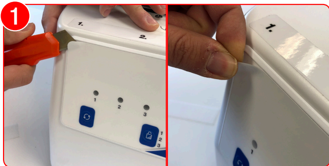
1 Peel off the damaged sticker
