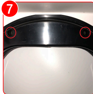
7 Flip the cabinet on its top and remove the two inner screws that are holding the lid tray assembly to the cabinet
