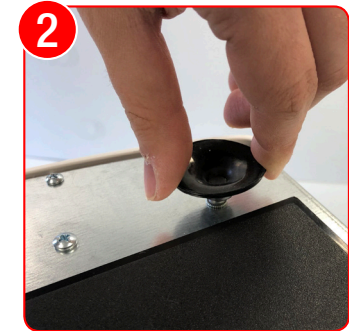
2 Screw the replacement foot/feet into the stud on the base of the centrifuge
