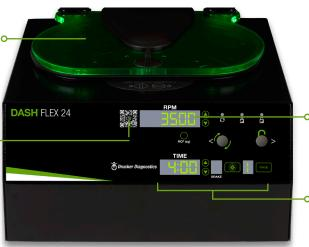
View RPM and remaining spin time on the digital display
