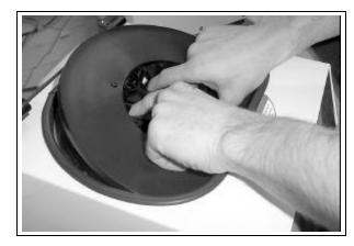
Proper Rotor Position for Installation and Removal
